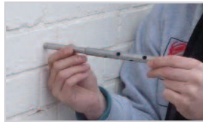
2. Fit the appropriate sized Load Test Key (LTK) at least 50mm (normally one full turn) over the end of the tie. Remove the cross pin, if fitted
