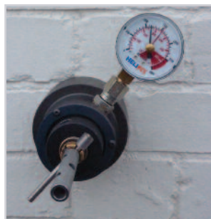
6. Note the reading and then release the tension on the tested wall tie
