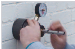
3. Slide the Load Test Unit (LTU) over the LTK and replace the cross pin, engaging it in the castellation on the top of the centre stud
